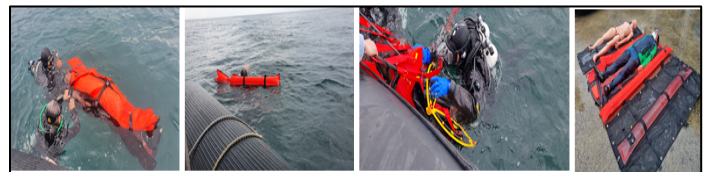
Figure 19: Experiments of SMB package, SMB detachable type, human lift buoyancy check.
