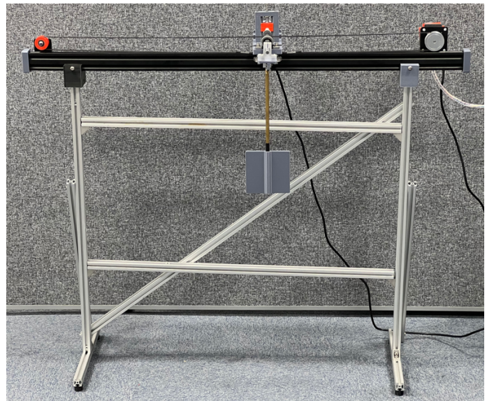
Figure 7: Pendulum mounted on its stand: The structure uses diagonal bracing to increase its rigidity.
