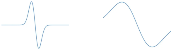
Figure 2: Squishing (left) or Stretching (right) by decreasing or increasing the value of 'a'
