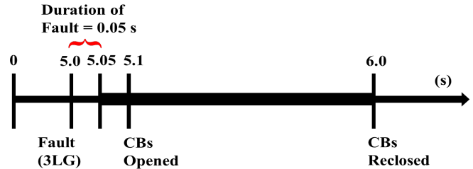
Figure 10: 3LG fault conditions.
