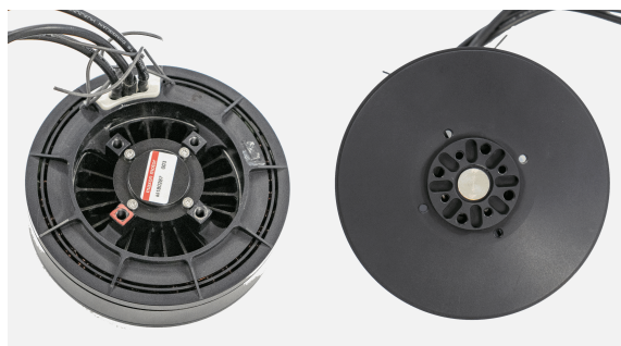
Figure 11: The test motor PMSM 1, UAV motor. On the back side, left, there are three thick motor power cables and four thin cables for two motor temperature sensors, which are applied for measurement of thermal behaviour later.
