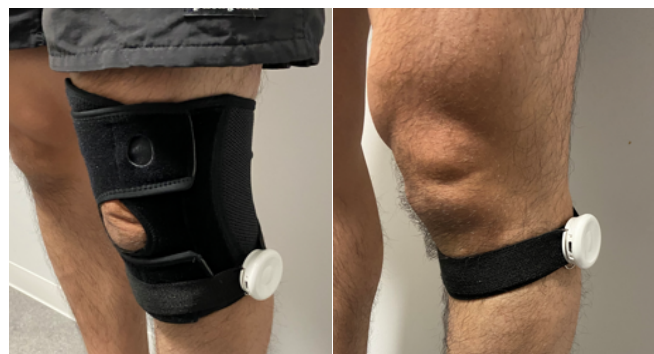
Figure 2: Placement of the accelerometer on the fibular head of the affected limb
