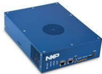
Figure 5. Real time embedded platform, Bluebox 2.0 by NXP
