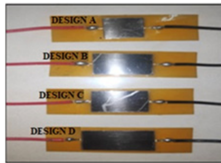
Figure 5: The completed fabrication of the FPVEH.
