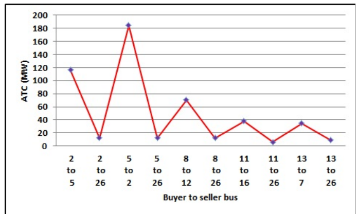
Figure 12: Variation of ATC values for all transactions due to generator at different buses
