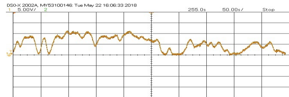
Figure 19: Real-time Indian City Drive Cycle at laboratory environment
