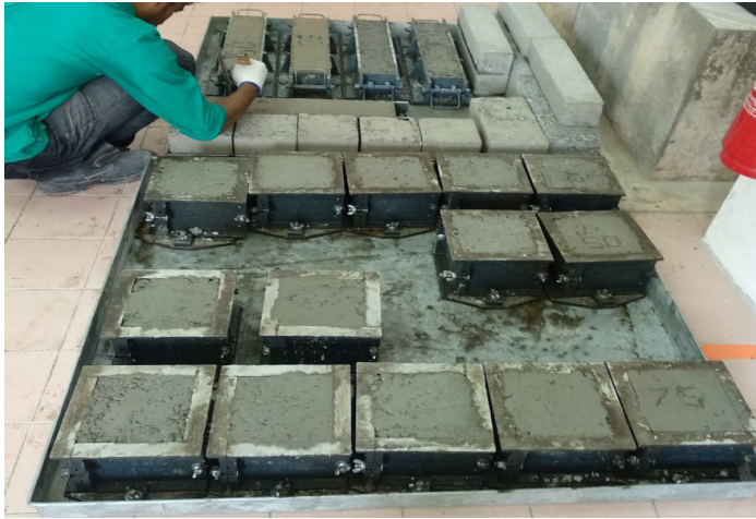
Figure 6: Concrete cubes and beams kept for 24 hours before curing
