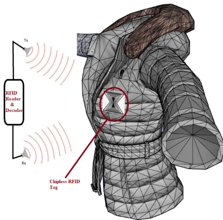
Figure 1: Structural diagram of Bow-Tie chip-less RFID system
