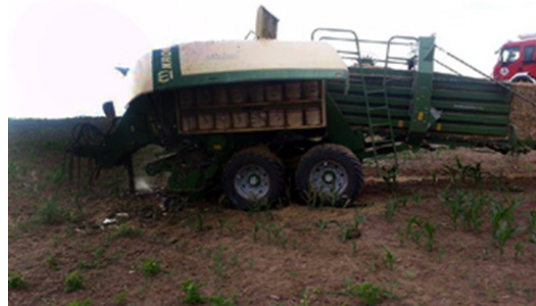
Figure 2: Damaged Big Pack 750 after the fire accident [10]
