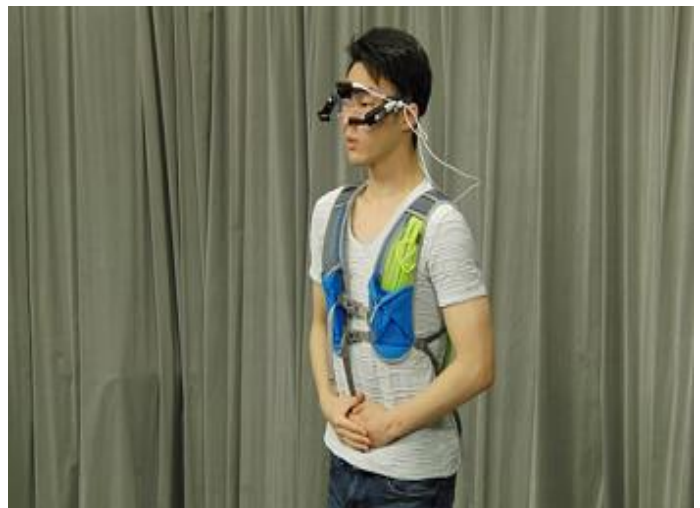
Figure 2: A person wearing the device (the eye movement measurement device is in the backpack)
