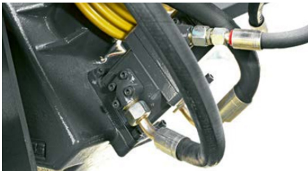
Figure 4: Two oil pumps supply the input gearbox and the TURBO FAN knot cleaning system with hydraulic oil. [14]
