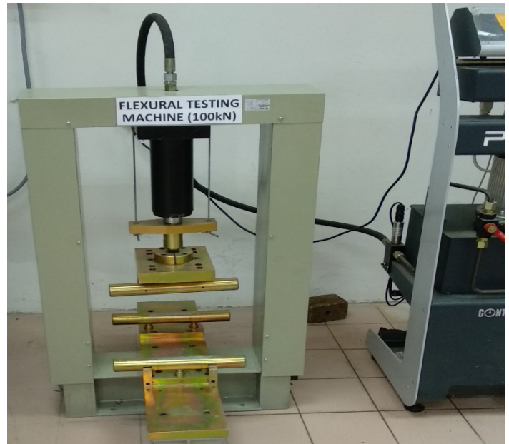
Figure 9: Flexural Testing Machine (Modulus of rupture Test)
