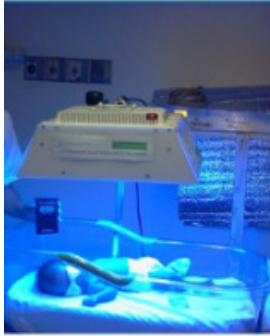
Figure 3: Low-cost Phototherapy Light System (LPLS)
