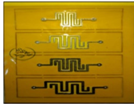
Figure 4: A fabricated IDE circuit.
