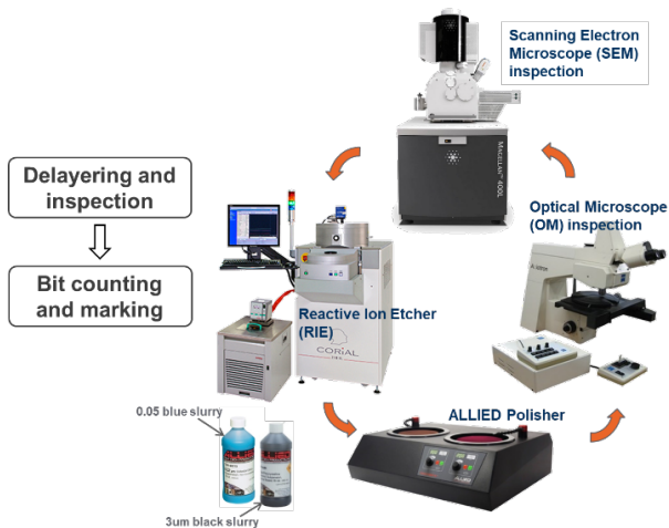
Figure 1: Illustration of typical PFA workflow for memory failure devices.
