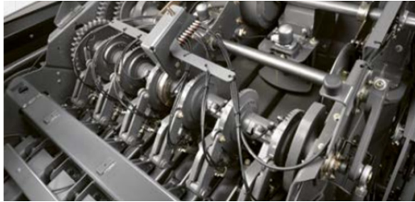
Figure 3: The hydraulically driven turbo fan system protects the knotters from pollution, a strong air flow with speed 140 km/h. [14]
