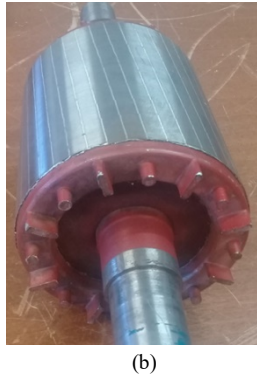
Figure 3: Photographs of prototype rotors (a) SynRM-BRBs (b) SCIM
