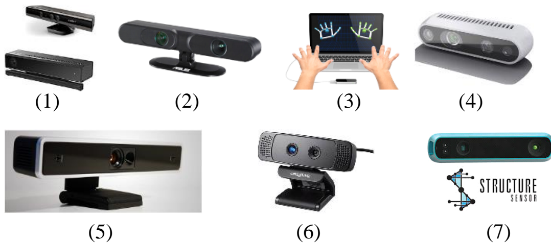
Figure 4: The depth sensor groups: (1) MS Kinect group; (2) ASUS Xtion group; (3) Leap Motion; (4) Intel RealSense group; (5) SoftKinetic group; (6) Creative Interactive Gesture; (7) Structure Sensor.
