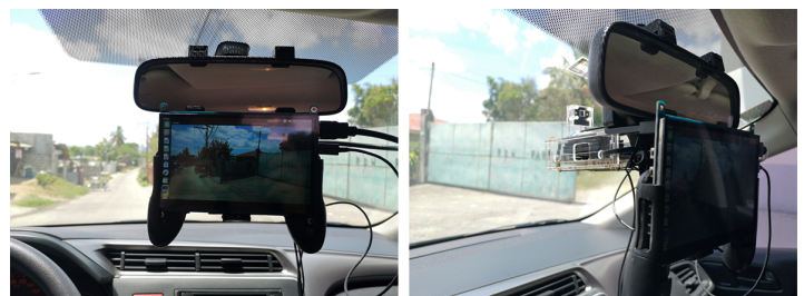
Figure 14: TSDR car setup for actual road testing
