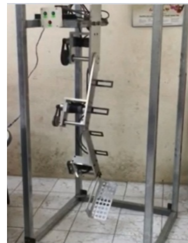
Figure 1: Mechanism of 3-DOF Rehabilitation Robot [1]
