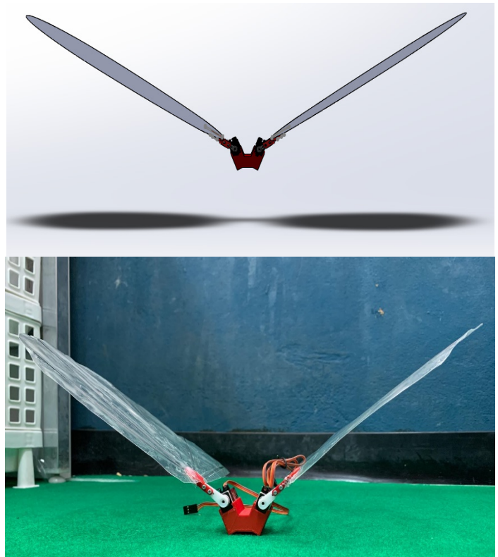
Figure 11: Butterfly robot model (top) and manufactured butterfly robot (bottom)
