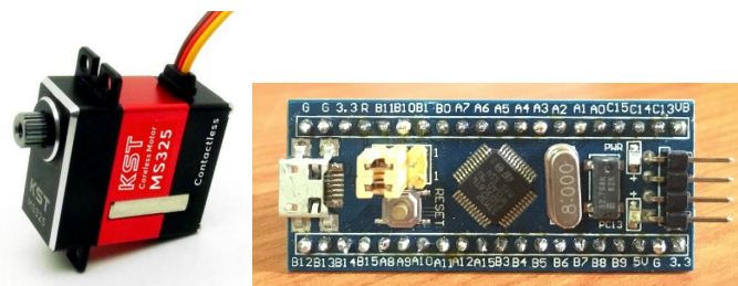
Figure 12: KST MS325 high speed servo (left) and ARM controller (right)
