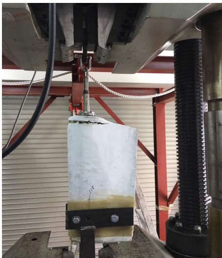
Figure 1. Broken wind turbine blade
