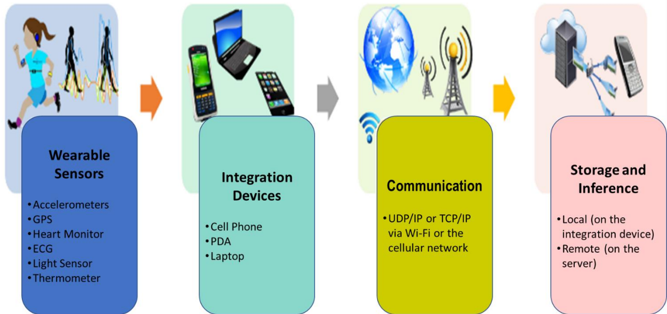
Figure 4: Generic data acquisition architecture for Proposed HAR systems
