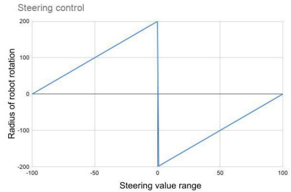
Figure 5: The varying values of D (Radius of robot rotation) according to the steering control (steering readings).
