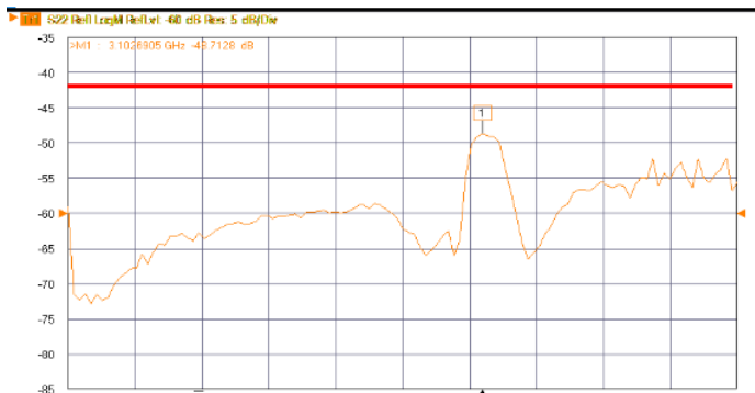
Figure 9 : PXIe-5632 Port 2 Directivity Validation Results Measured from 300 kHz to 5 GHz
