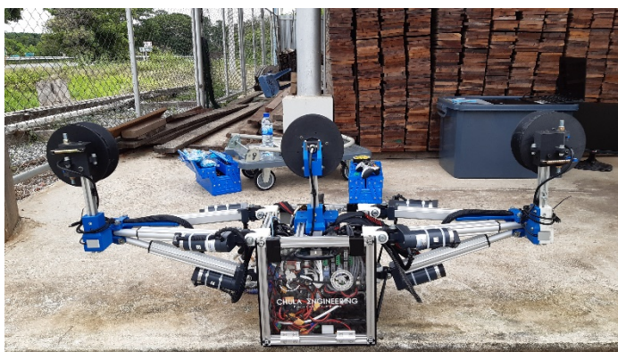
Figure 19: The developed inspection robot during set-up before the field test
