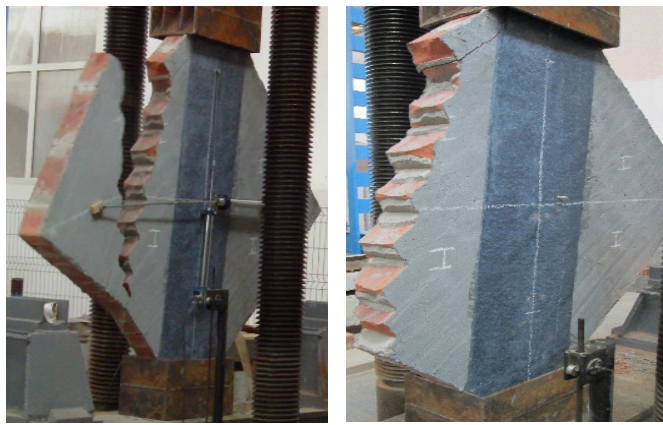
(a) Shear cracking (Side I)
