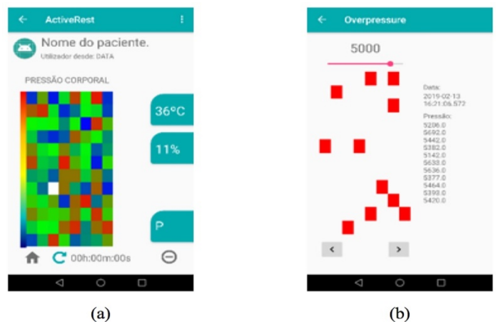
Figure 7: Android App screenshots: (a) the main page where the data from the pressure mapping, and the temperature and humidity values are shown, as well as the repositioning timer, and (b) the page with the history of critical pressures that exceed the established threshold.
