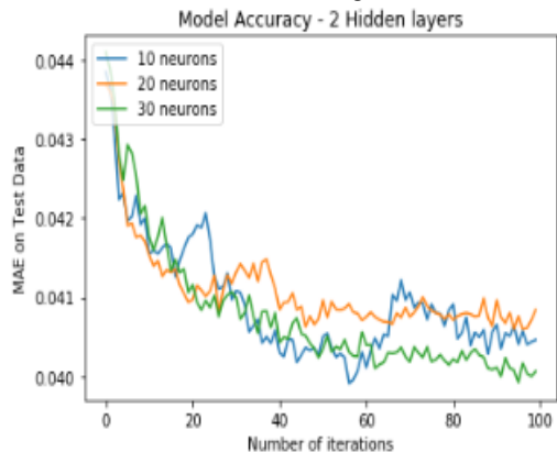
Figure 5: MAE of LSTM with 2 hidden layers for 24-hour time lag
