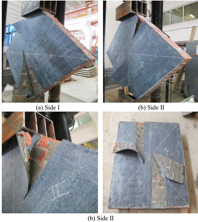
Figure 5: Failure mode of W- CFRP-W 1
