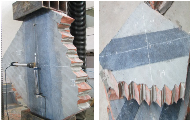
(b) Shear cracking (Side II)
