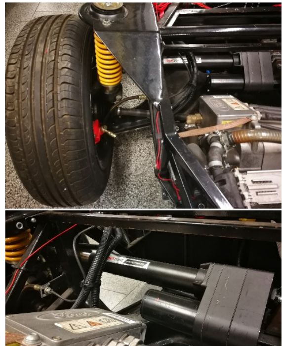
Figure 11 – Picture of testing vehicle with steer-by-wire technology
