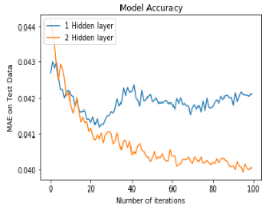
Figure 6: MAE with 1 and 2 hidden layer, each having 30 neurons each for 24 hour time lag
