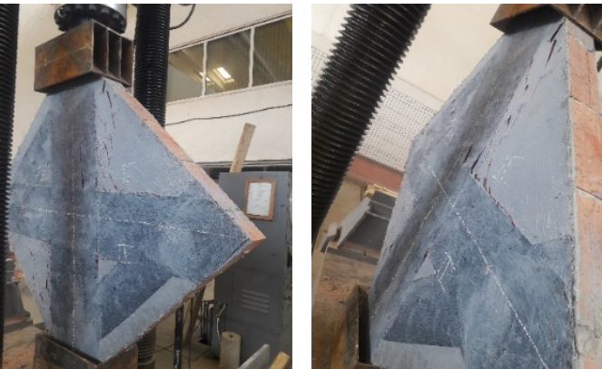
(b) Delamination and shear cracking (Side II)
