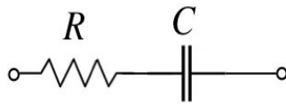
Figure 3: Used configuration of the varactor model depending on resistance R and capacitance C implemented in series.
