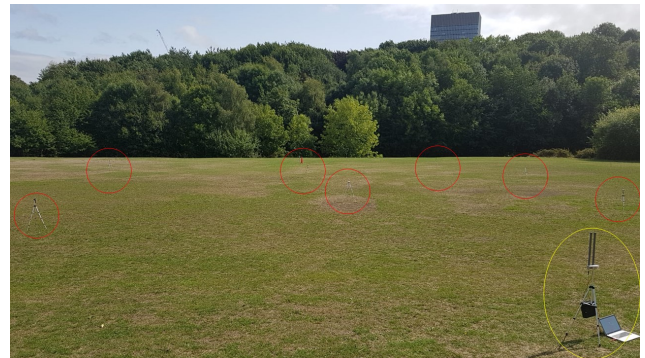
Figure 9: Outdoor experimental setup showing some of the distributed users on red and deployed observer system on yellow
