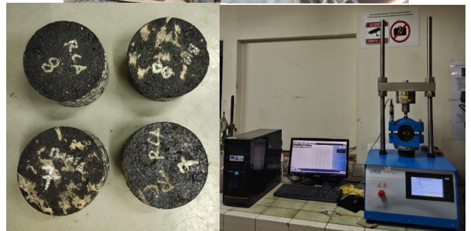
Figure 10: Molding of Marshall test samples from APB samples
