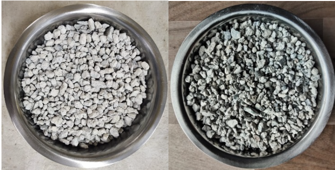
Figure 4: RCA granules before and after the washing process
