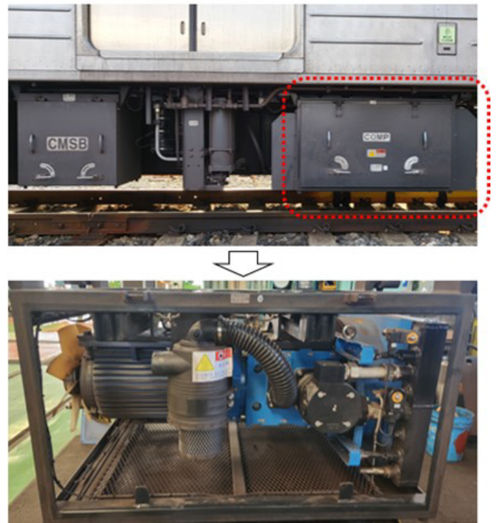
Figure 4: Air compressor of the Electric multiple unit
