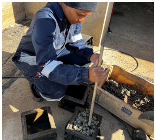
Figure 12: Compacting with a rod.
