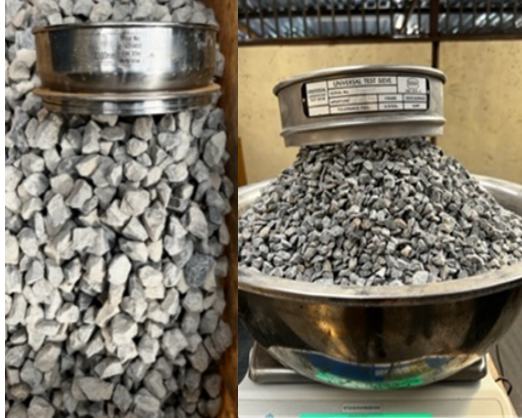
Figure 7: Laboratory sieved and weighed Material and labelled according to size.
