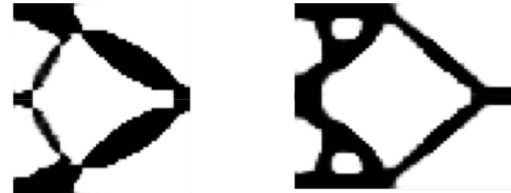
Figure 12: Optimized force inverter with different objective functions. Left: use geometry advantage; Right: use target displacement
