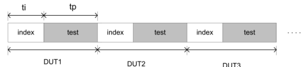
Figure 2: Testing time of DUT consists of index time t_i and test time t_p
