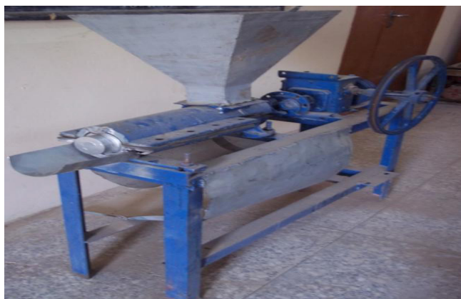
Figure 7: Image of a multi Fruit juice Extractor [15]
