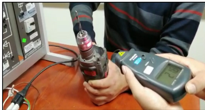
Figure 6: Analysis of the motor with the application of an Alternate Voltage.
