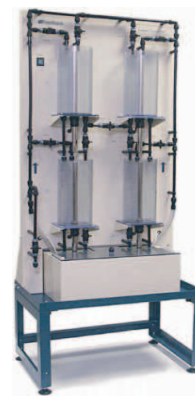
Figure 6: Plant of four coupled tanks [26]
