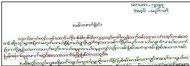
Figure 16: Text line segmentation of Gradient Magnitude with Anisotropic Gaussian on scale (2, 1)
