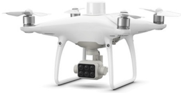
Figure 2: UAV used for monitoring (Phantom 4 Multispectral)
