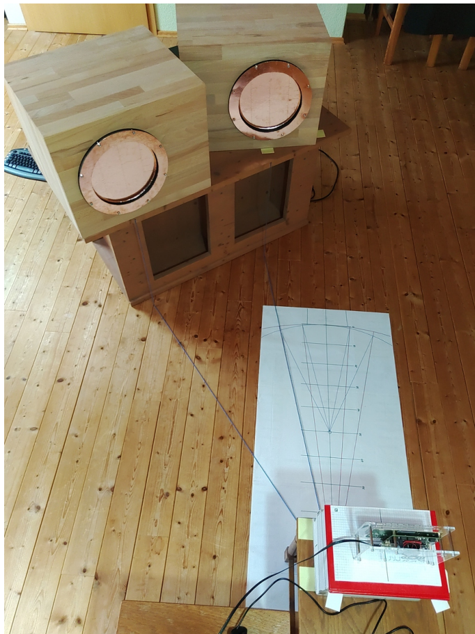
Figure 12: Picture of the measurement setup to investigate dynamic clutter with two loudspeakers.
