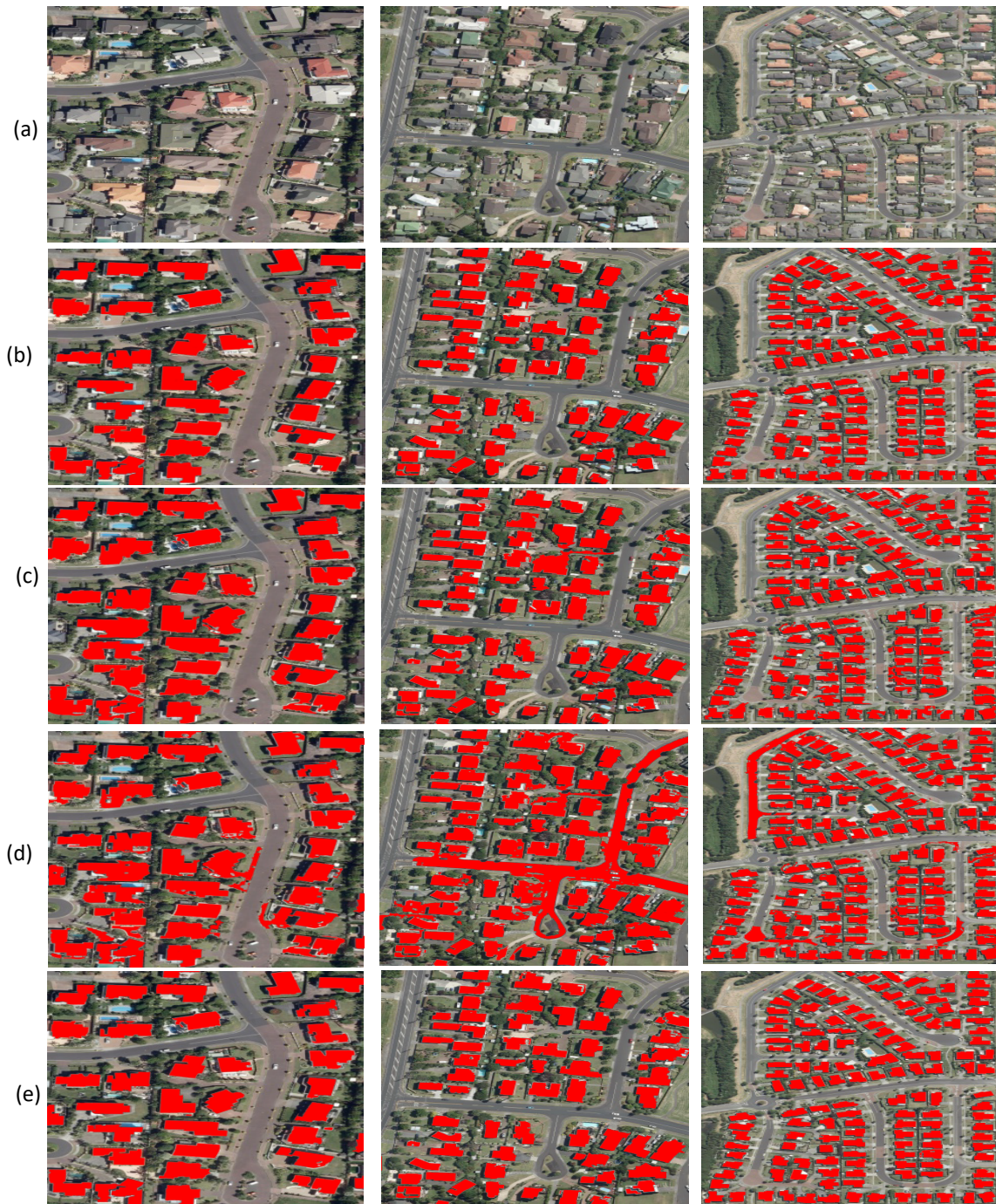
Figure 5: Comparison of building detection results obtained by three different algorithms where (row a) Test images, (row b) The results of the proposed method, (row c) The results of the method [15], (row d) The results of the method [23] and (row e) The results of the method [26]. (Red represents building results).
