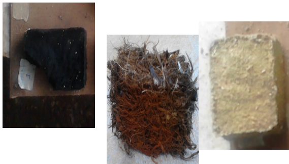
Figure 3: Pure briquettes of coal, palm mesocarp fibre (pmf) and corn cob.
