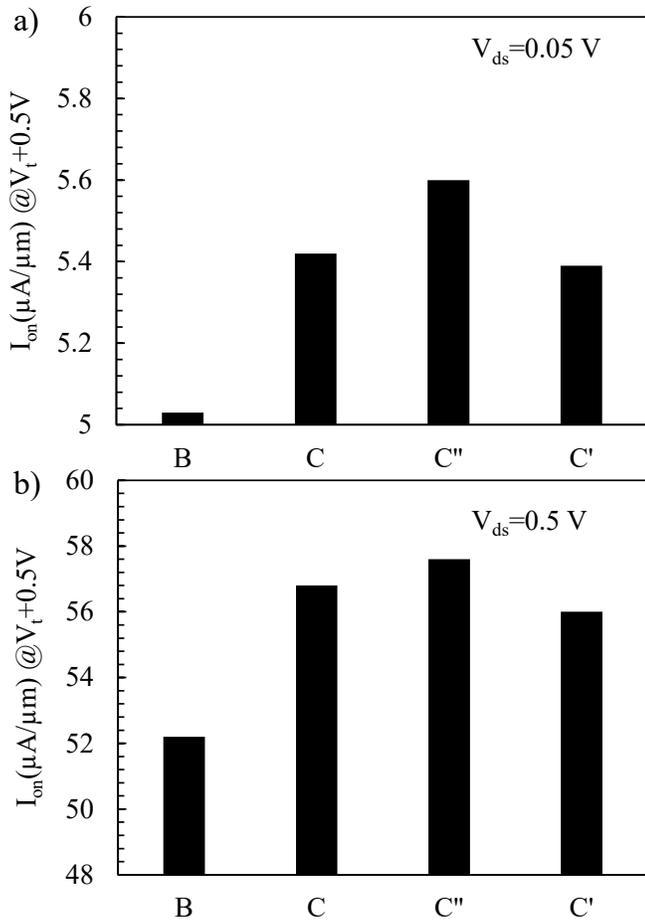
Figure 16:  $I_{on}$  extracted at  $V_t+0.5V$  and for  $V_{ds}=0.05V$  (a) and  $V_{ds}=0.5V$  (b),  $W$  of the devices =  $100\mu m$ ,  $L_g=10\mu m$ . Replacement of  $Al_2O_3$  (B) by  $LaSiO_x$  (C) in the gate stack improves  $I_{on}$ . Further improvement can be seen when the gate stack is scaled down ( $C''$ ).
