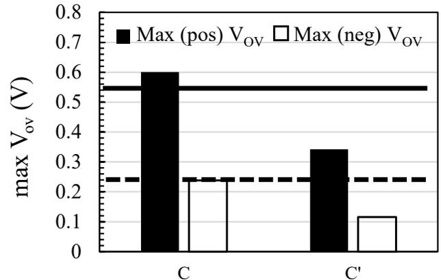
Figure 11: Max  $V_{\text{ov}}$  measured from positive and negative CV-BTI on MOS capacitors. For a target  $V_{\text{DD}}=0.8$  V, the max pos  $V_{\text{ov}}$  target (full line) is  $0.53$  V and the max neg  $V_{\text{ov}}$  target (dashed line) is  $-0.26$  V (i.e.  $1/3*V_{\text{DD}}$ ).
