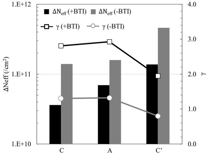
Figure 20  $\Delta N_{\text{eff}}$  and  $\gamma$  extracted from BTI measurements on MOSFETs applying both positive and negative stress conditions. The data from MOSFETs confirm the trends observed on MOSCAPs.
