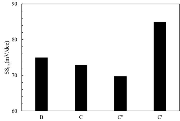
Fig. 17  $SS_{lin}$  for various gate stacks.  $L_g=50\mu m$ .  $SS_{lin}$  reduces by replacing  $Al_2O_3$  (B) with  $LaSiO_x$  (C) in the gate stack. Scaling the  $HfO_2$  ( $C''$ ) thickness leads to further reduction.
