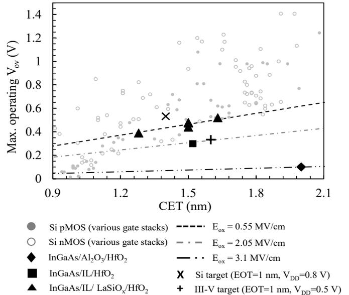
Figure 22. Max. operating overdrive voltage as a function of CET for various gate stacks on Si (p- and n-MOS) and InGaAs. The devices with the IL/LaSiO<sub>x</sub>/HfO<sub>2</sub> gate stack surpass the reliability target for III-V semiconductor based technology.
