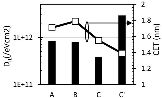
Figure 7: Mid gap  $D_{it}$  (bars) and CET (dots) extracted from the C-V data presented in fig. 6. Replacement of  $Al_2O_3$  (B) by  $LaSiO_x$  (C) reduces the  $D_{it}$  to less than  $4 \times 10^{11}/cm^2.eV$ . The CET drops to 1.55 nm.
