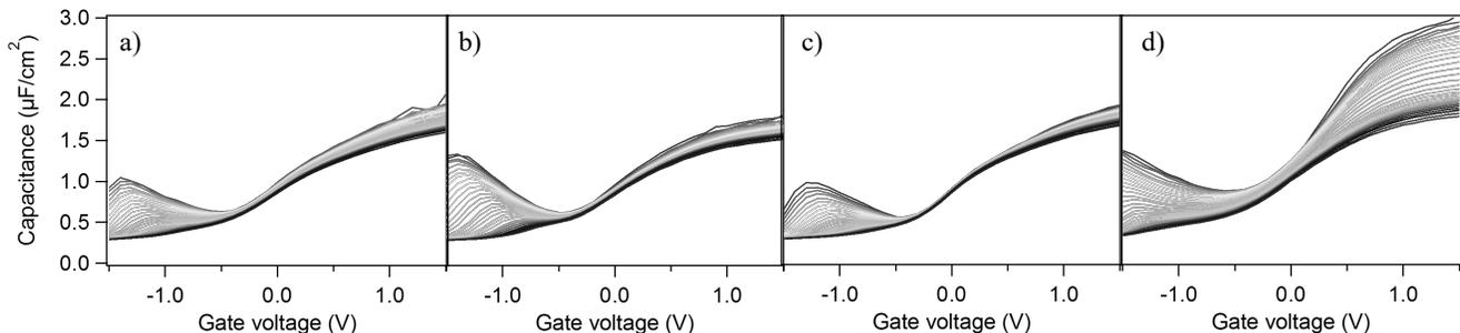
Figure 6. RT MF-CV's measured from dot capacitors of A) 1 nm IL/3 nm  $HfO_2$ , B) 1 nm IL/1 nm  $Al_2O_3$ /3 nm  $HfO_2$ , C) 1 nm IL/1 nm  $LaSiO_x$ /3 nm  $HfO_2$ , C') 1 nm  $LaSiO_x$ /3 nm  $HfO_2$ . Frequencies between 1 kHz-1 MHz (red-blue) were measured with logarithmic spacing. All capacitors received a PMA in forming gas for 5 minutes.
