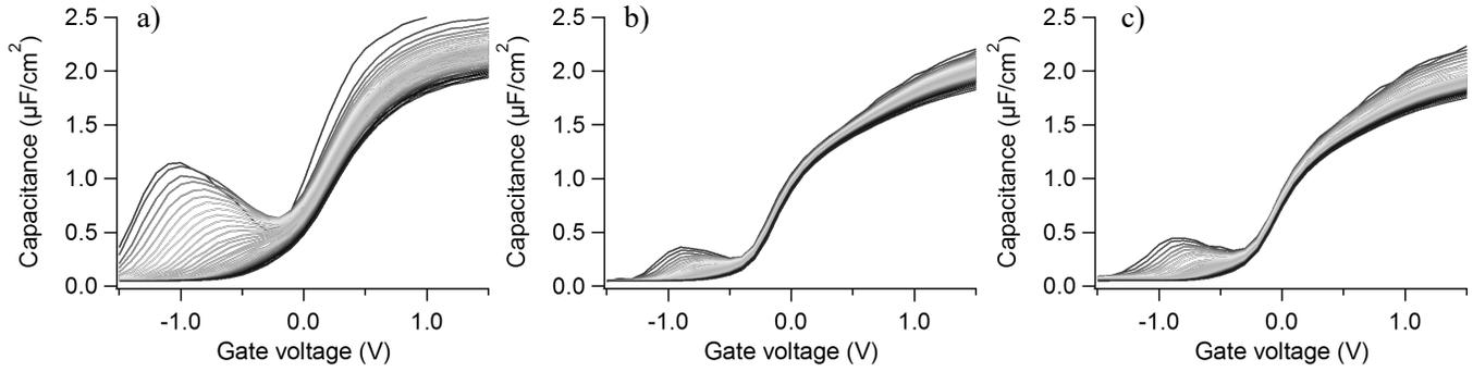
Figure 3. Measured RT CV's of gate stacks a) 'ref', b) A and c) B' described in Table I at 31 frequencies between 1kHz and 1MHz. The MOSCAP devices received a PDA at 400°C, 5' in Forming gas.
