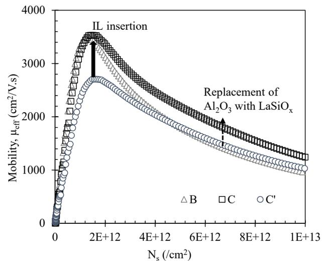
Figure 19 Improvement in the mobility at low  $N_s$  (due to the introduction of IL) and high  $N_s$  (as a result of replacement of  $Al_2O_3$  with  $LaSiO_x$ ). Mobility was extracted from  $L_g=50\mu m$  devices.
