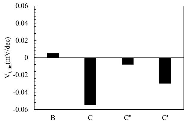
Figure 18  $V_{t,lin}$  for various gate stacks.  $L_g=50\mu m$ . Slight  $V_{t,lin}$  reduction by replacing  $Al_2O_3$  (B) with  $LaSiO_x$  (C) in the gate stack is observed.
