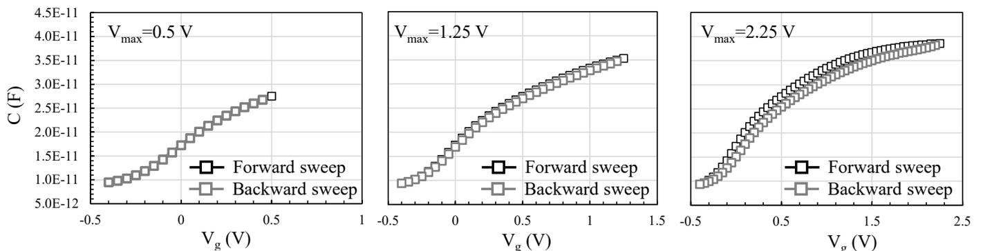
Figure 9. 100 kHz CV up and down traces of the  $1$  nm IL/ $1$  nm  $\text{LaSiO}_x$ / $3$  nm  $\text{HfO}_2$  gate stack measured at 3 different  $V_{\text{max}}$ .  $V_{\text{start}}$  was  $V_{\text{fb}}-0.5$  V.
