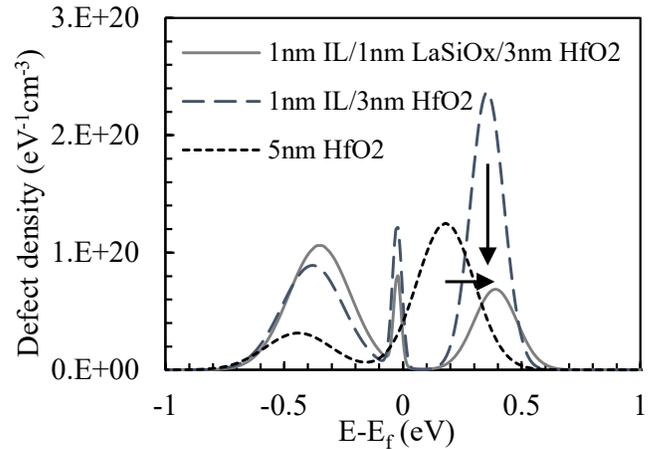
Figure 13: Defect density profile obtained by modeling the  $\Delta V_{th}$  vs  $V_{gate}$  as described in [25]. Insertion of the IL layer causes narrowing of the shallow defect band, thus enhancing  $\gamma$  and shifting the mean defect level of this band to shallower energy [19] but increases the density of defects at deeper energies. Insertion of  $LaSiO_x$  consistently reduces the total defect density (both shallow and deep energies).
