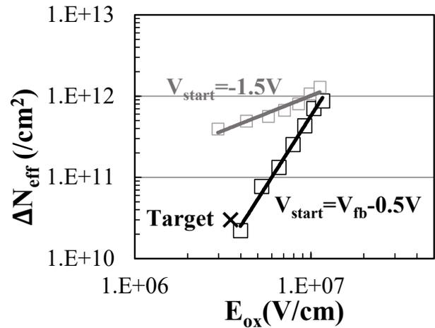
Figure 10:  $\Delta N_{\text{eff}}$  as a function of applied  $E_{\text{ox}}$  for the stack with  $1$  nm IL/ $1$  nm  $\text{LaSiO}_x$ / $3$  nm  $\text{HfO}_2$  for 2 different  $V_{\text{start}}$  conditions.  $V_{\text{start}}=-1.5$  V and  $V_{\text{start}}=V_{\text{fb}}-0.5$  V. The large dependence on the  $V_{\text{start}}$  conditions points to the presence of deep traps i.e. located at energies below InGaAs  $E_f$  at flatband.
