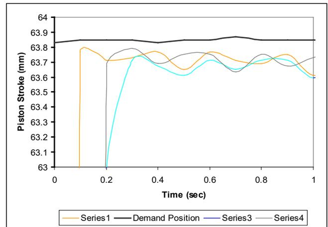
Figure. 5. The system performance focused around target position
