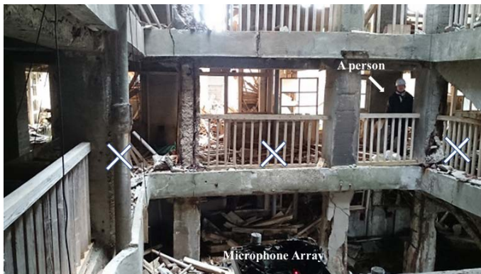
Figure 8: Experimental scenario using falling cans and stones that hit the second floor of the building as sound sources
