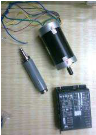
Figure 1: The analysed BLDC motor (stator, rotor) with PWM converter for power supply
