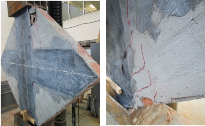
(b) Delamination and shear cracking (Side II)
