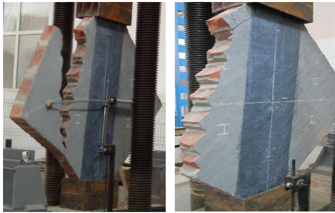
(a) Shear cracking (Side I)
